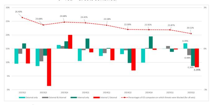
The diagram shows that the decrease in the percentage of attacked ICS computers in Q2 2025, against the backdrop of growth in the set of external threats, was driven by a decline in the percentage of attacked ICS computers belonging to the borderline set and the set of internal threats.
